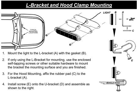
Once installed, have someone stand 20 feet in front of the vehicle to view the lights. Adjust them as needed and fully tighten the Phillips head screws on each light.
