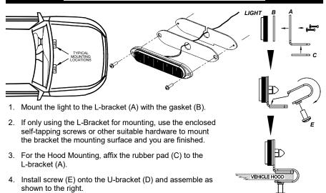
Once installed, have someone stand 20 feet in front of the vehicle to view the lights. Adjust them as needed and fully tighten the Phillips head screws on each light.
